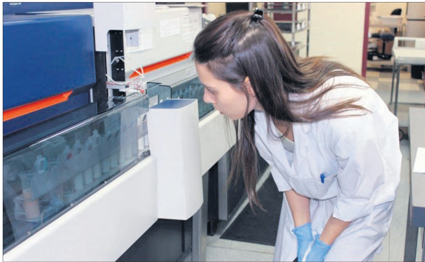
The latest generation of infrared analyzers now in use in Valacta's laboratories can, with proper calibration, produce a summary milk fatty acid profile very quickly and at much less cost.
