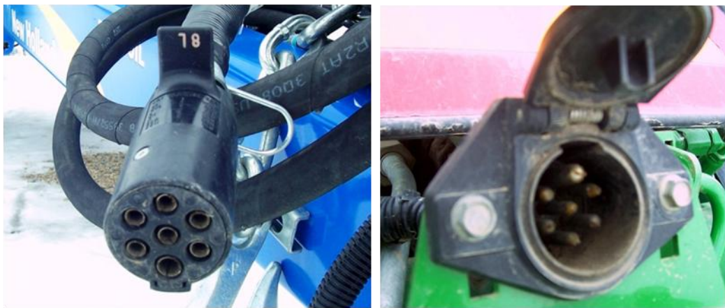
Implement Plug (male) and Tractor Receptacle (female) Seven-Conductor Electrical Connector
